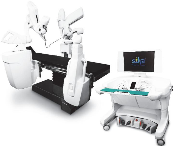
Figure 1 – The Sina<sub>flex</sub> robotic telesurgery system
