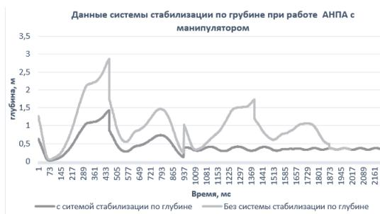
Figure 2 – The work of the depth stabilization system of the apparatus during the operation of the MC
