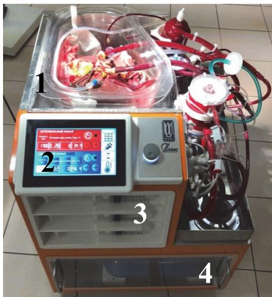
Figure 1 – General scheme of the components of a PC DO (front view): 1 - a container for fixing and connecting a donor organ, 2 - a display for controlling parameters, 3 - volumetric infusion pump, 4 - a portable oxygen source
