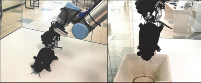
Figure 1 – Different configurations of anthropomorphic hand when manipulating an object
