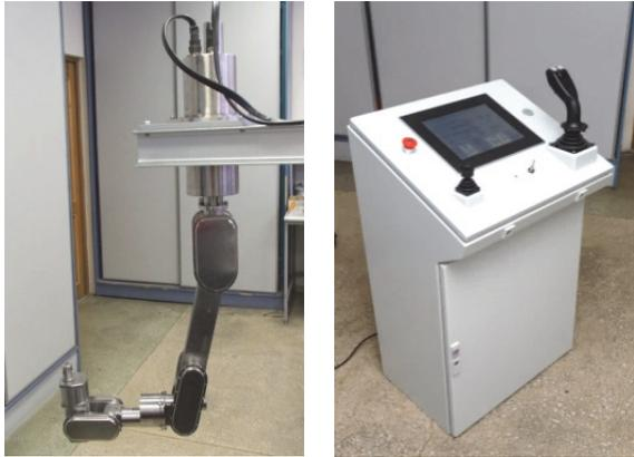
Figure 1 – General view of manipulator MR-48 and its control station
