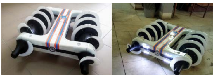
Figure 2 – The running model of a single segment of the multi-jointed robotic platform
