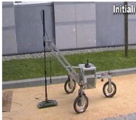
**COMMERCIAL WHEELED ROBOT:** finally we opted for the se of a commercial platform (called ROBUDEM)
